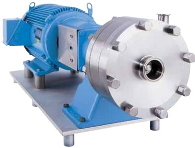
SPX offers three single stage and one multistage high-pressure 200 Series centrifugal pump models. Designed for use in membrane filtration systems (reverse osmosis and ultra filtration), they can accommodate high system pressure inlet conditions to 1000 PSI producing a smooth, pulse-free high discharge pressure for reduced membrane wear and increased product quality.
